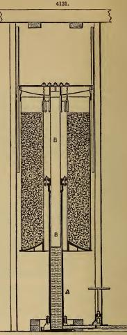
pressure of water for practical use seems to be that mentioned above, namely, 1500 ft. or about 700 lbs. a square inch. By increasing the pressure the size of the pipes and of all parts of the appa-
